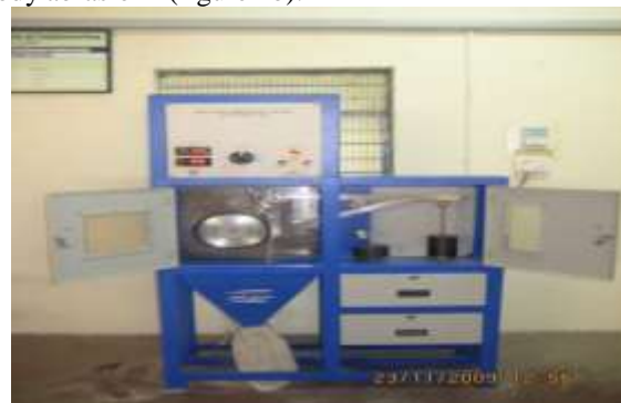
Figure 3: Dry sand abrasive wear testing machine
